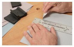
Using a rigid straight edge, align it to the first set of marks you made on the sandpaper sheet. Once the straight edge is in place, hold it down firmly and slowly start tearing the strip of sandpaper until you create an 11" strip.
