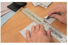
Lay your straight edge across the fold line and hold it firmly in place. Tear the sandpaper along the fold line while holding the straight edge.
